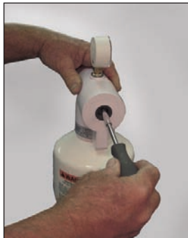
FIGURE 6. Turn the adjustment screw.
