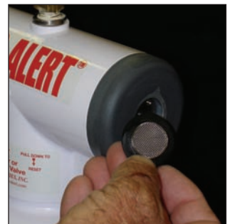
FIGURE 3. Remove the vent screen.
