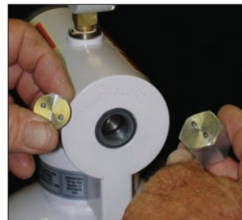
FIGURE 2. Remove security cap with the spanner tool.
