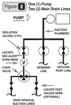
A: Always Locate The Vac-Alert <sup>™</sup> SVRS On The Main Drain Suction Line. SVRS Unit Must Be Mounted In The Vertical Position.
