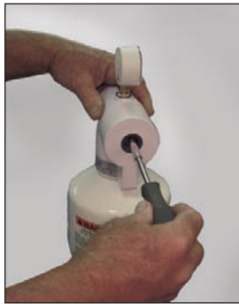
FIGURE 6. Turn the adjustment screw.
