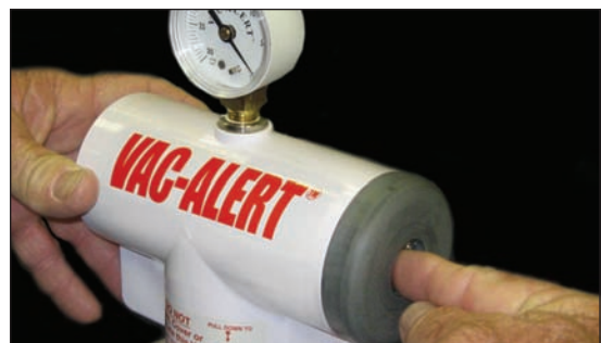
FIGURE 4. Test for an air leak by tapping the vent hole (the gray end of the SVRS unit).
