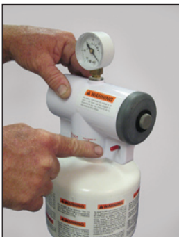
FIGURE 7. Reset lever. In the up position before being reset, and the down position after being reset.
