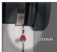
FIGURE 7. Reset lever. In the up position before being reset, and the down position after being reset.
