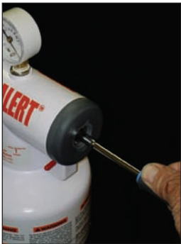
FIGURE 5. Lock open the piston.
